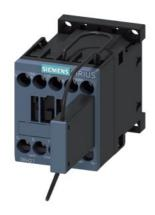
Contactor relay railway, 2 NO + 1 NC, 110 V DC, 0.7 ... 1.25\* US, with integrated suppressor diode, Size S00, screw terminal installation on standard mounting rail optimized (20 G) suitable for PLC outputs
