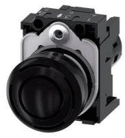
acoustic signal device, compact, 22 mm, round, plastic, black, Continuous tone 2.4 kHz, IP40, Sound pressure min. 80 dB/10 cm, with holder, Operating voltage 24 V AC/DC, screw terminal
