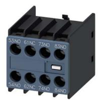
auxiliary switch, on the front, 3 NO + 1 NC, 53/54, 61/62, 73/74, 83/84, current path: 1 NO, 1 NC, 1 NO, 1 NO, screw terminal, physically coded, only with contactor relays 3RH2140 and 3RH2440 combinable (according to EN 50011)
