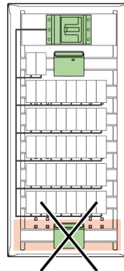
Illustration 6: NSX/NSXm on a mounting plate at the top of the W600/W850 (With or without incoming connection block)
