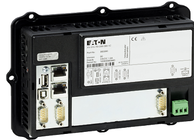
Fig. 9: Service side with optional interfaces XV-313-70-...
