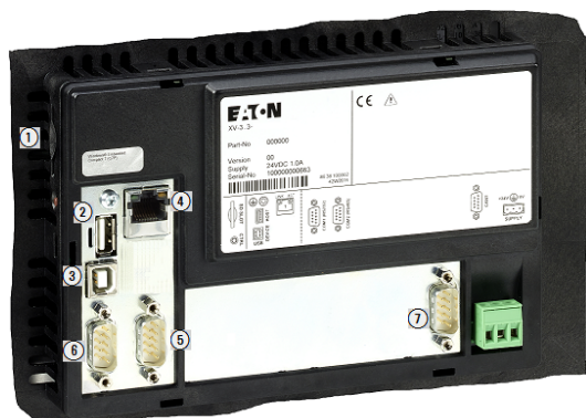
Fig. 24: Basic interfaces on all HMI-PLC units
