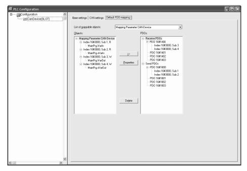
The **Default-PDO-Mapping** tab allows the entries which are defined in the Parameter Manager to be assigned/modified to the "Mapping" of the CAN-Device.
