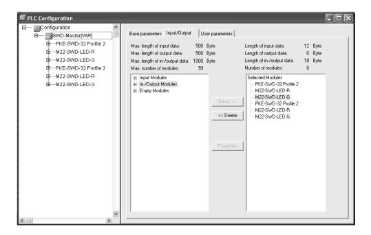
Clicking the **Properties** button opens the Module Properties dialog of the currently selected SmartWire-DT slave. It shows the name, the Config (coding of the IO image in accordance with the PROFIBUS standard) and the input and output length of the module in bytes.
