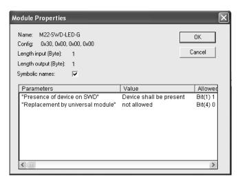
The parameters 'Presence of device on SWD' and 'Replacement by universal module' are standard parameters for all SmartWire-DT slaves.
