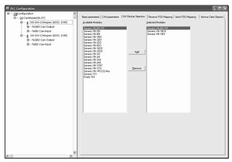
If the inserted CAN module has a modular design and if it supports the appropriate standards (**DSP 301, V4.01 and DSP 306**), then the tab **CAN Module selection** appears. The configuration of the appropriate structure can be made by adding with **Add** button or removing with **Remove** button.
