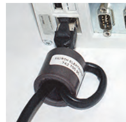
Figure 7: Ethernet cable shielding example: double loop through ferrite core
