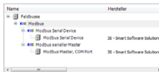
Figure 97: Adding a Modbus device
