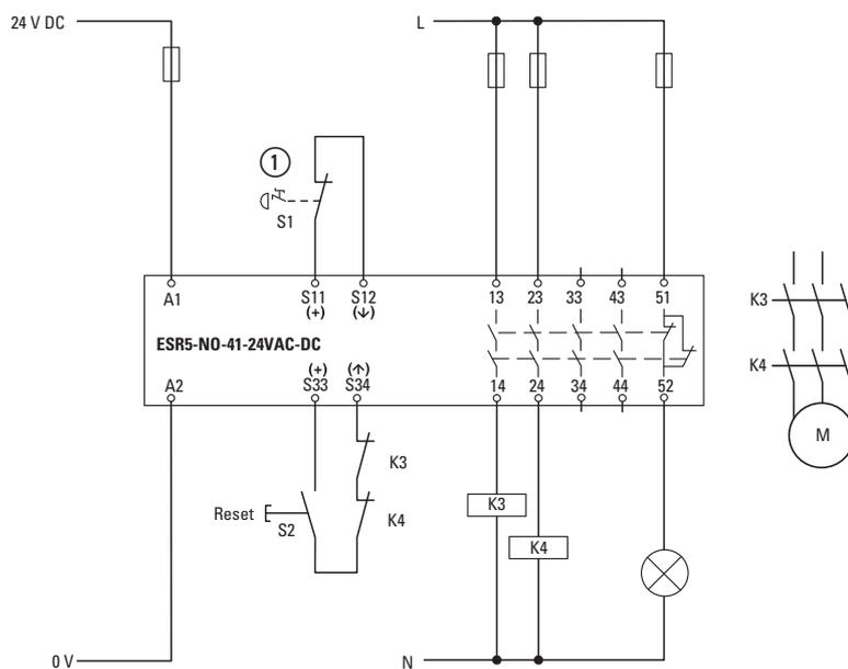
Figure 12: Single-channel emergency stop monitoring/manual start
