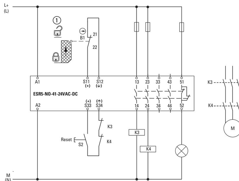
Figure 11: Single-channel safety door monitoring/manual start
