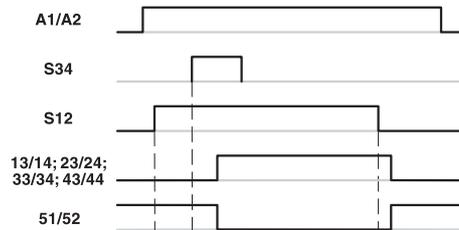
Figure 6: Time diagram for manual start
