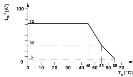
Figure 3: Derating curve - vertical or horizontal mounting position, without spacing
