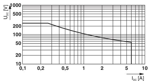
Figure 4: Relay load curve - ohmic load
