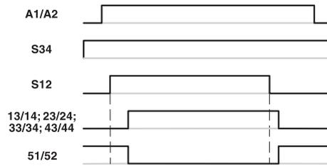
Figure 5: Time diagram for automatic start
