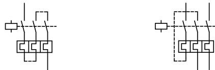
Figure 4: Wiring of the overload relay for the protection of AC or DC motors (bimetallic releases wired in series)
