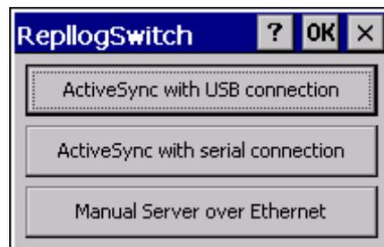
The «Repllogswitch.exe» program is used for establishing a connection with a PC via «ActiveSync» or «Manual Server». This is described in the chapter [Procedure: ActiveSync](#) or [Procedure: Manual Server](#).
