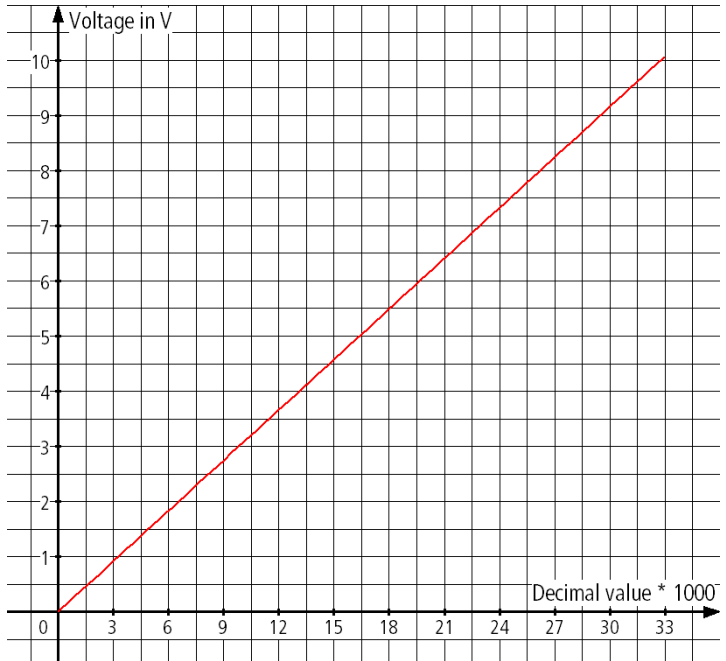
Figure 28: Representation of voltage values in relation to the decimal values in the coordinate system
