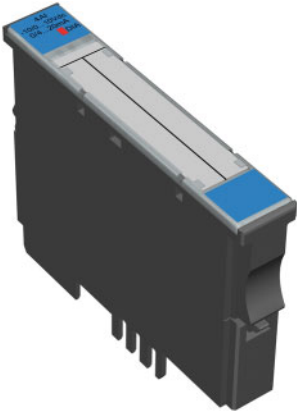
Figure 70: Analog input module, 4 analog inputs: voltage (-10...+10 V DC/0...+10 V DC) / current (0...20 mA/4...20 mA)
