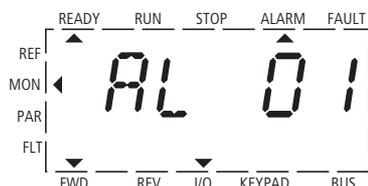
Figure 118: Example of an alarm message
