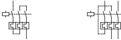
Figure 8: Wiring of the motor-protective relay for the protection of AC or DC motors (bimetallic release switched in series)
