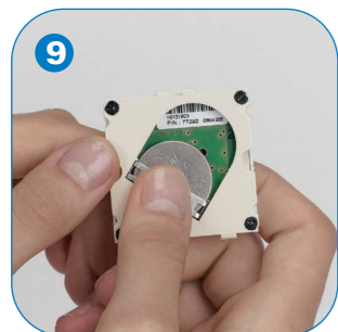
9 Battery easy to replace. Service life of battery for push-button approx. 10 years
