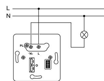
**Insert with mechanical push-button via PlusLink**
