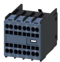
auxiliary switch, on the front, 2 NO + 2 NC, 11 U, 53/54, 61/62, 75/76, 87/88, current path: 1 NO, 1 NC, 1 NC (lagging), 1 NO (leading), spring-loaded terminal, for contactors 3RT2 and contactor relays 3RH2
