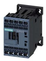
Coupling contactor relay, 4 NO, 110 V DC, 0.7  $\dots$  1.25\* US, with integrated suppressor diode, Size S00, Spring-type terminal suitable for PLC outputs
