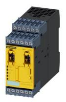
Fail-safe digital module DM-F local, for fail-safe shutdown via hardware signal Us: 110...240 V AC/DC 2 relay enabling circuits, 2 relay outputs, safety function can be set via DIP switch, maximum achievable SIL IEC 61508: 3, maximum achievable PL ISO 13849-1: E
