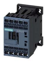
Contactor relay for railway 4 NO DC 72-125V, 0.7...1.25\*US, with integrated varistor Size S00, Spring-type terminal suitable for PLC outputs
