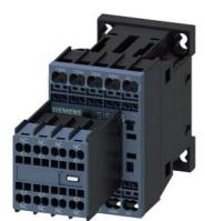
Contactor relay, 4 NO + 4 NC, 110 V AC, 50 / 60 Hz, Size S00, spring-type terminal, Removable auxiliary switch
