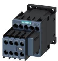
Contactor relay, 5 NO + 3 NC, 240 V AC, 50 / 60 Hz, Size S00, screw terminal, 2 NO + 2 NC basic unit / EN Varistor plugged on
