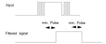
In bounce rejection mode, the system delays all transitions until the signal remains stable for the duration defined for the filter level.
