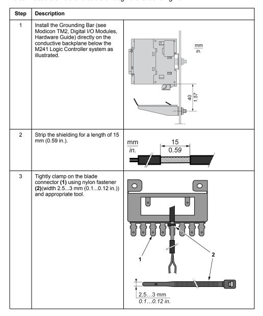
**NOTE:** Use the TM2XMTGB Grounding Bar for Functional Ground (FE) connections.
