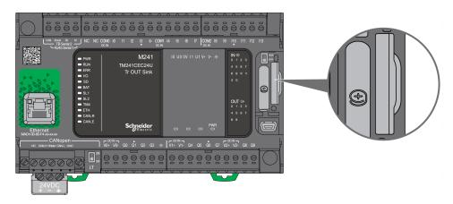
It is possible to set the Write-Control Tab to prevent write operations to the SD card. Push the tab up, as shown in the example on the right-hand side, to release the lock and enable writing to the SD card. Before using an SD card, read the manufacturer's instructions.
