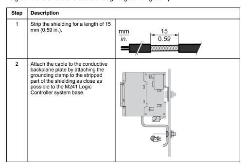
**NOTE:** The shielding must be clamped securely to the conductive backplane to ensure a good contact.
