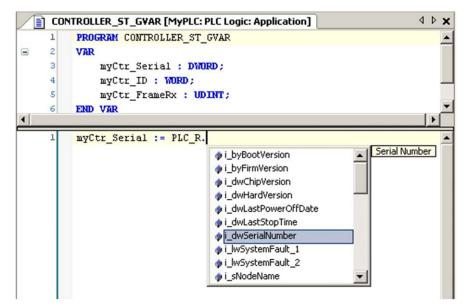
**NOTE:** In the example above, after you type the structure name  $PLC_R$ , EcoStruxure Machine Expert offers a pop-up menu of possible component names/variables.
