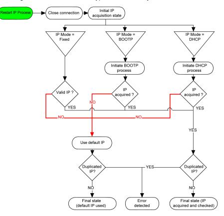
This diagram shows the different types of address systems for the controller:
