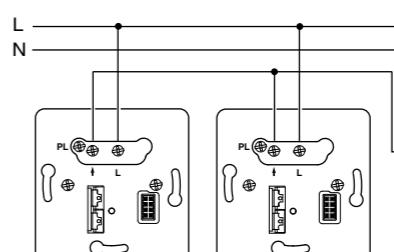
**Insert with mechanical push-buttons via PlusLink**
