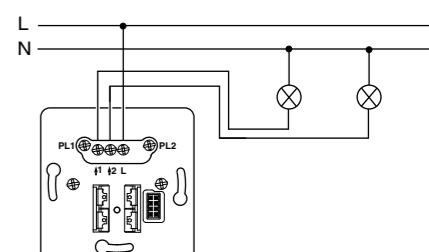
**Insert with mechanical push-buttons via PlusLink**
