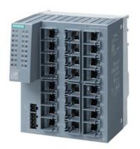
SCALANCE XC124, Unmanaged IE switch, 24x 10/100 Mbit/s RJ45 ports, LED diagnostics, error-signaling contact with set pushbutton, redundant power supply Manual available as a download .
