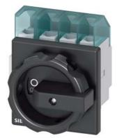
SENTRON, Switch disconnector 3LD, main switch, 4-pole, lu: 25 A, Operating power / at AC-23 A at 400 V: 9.5 kW, front-mounted, rotary operating mechanism, black, 4-hole mounting of the handle
