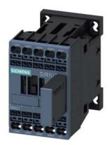
Coupling contactor relay, 4 NO, 24 V DC, 0.85  $\dots$  1.85\* US, with varistor plugged on, Size S00, Spring-type terminal
