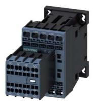
Contactor relay, 7 NO + 1 NC, 24 V DC, with integrated diode Size. S00, spring-type terminal, Removable auxiliary switch
