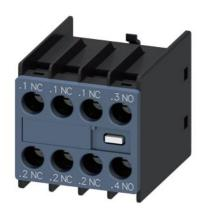
Auxiliary switch on the front, 1 NO + 3 NC Current path 1 NC, 1 NC, 1 NC, 1 NO for 3RH and 3RT screw terminal .1/.2, .1/.2, .1/.2, .3/.4
