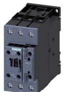
power contactor, AC-3 51 A, 22 kW / 400 V 1 NO + 1 NC, 230 V AC, 50 Hz, 3-pole, size S2, screw terminal
