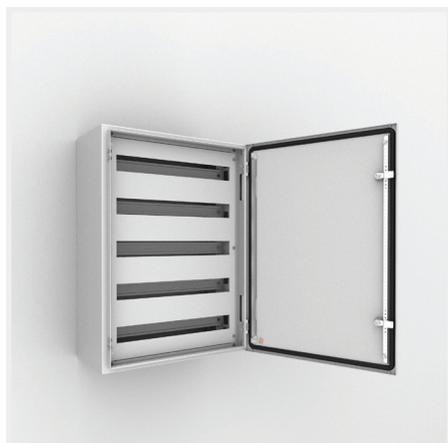
**Omschrijving:** Used for easy mounting of DIN-rail components with a maximum height of 68 mm. Distance between rows 125 mm. If required, the standard enclosure door can be replaced with a glazed door. Usable depth between front cover and external door: 35 mm. In stainless steel enclosure machining is required.
