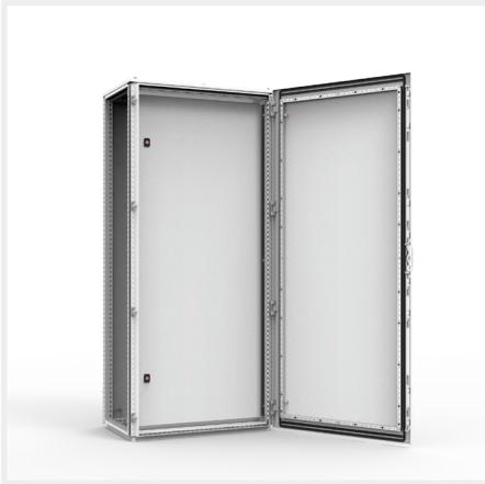
**Omschrijving:** Inner door provides a hinged mounting surface for equipment behind a standard or glazed front door. A mounting space of 80 mm, is available between the doors when the inner door is in the forward position. Can be adjusted in depth by steps of 25 mm. The mounting plate remains usable behind the inner door. The door is equipped with two double-bit 3 mm locks, and plastic handles.
