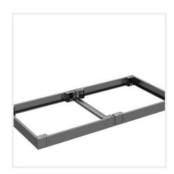
**Omschrijving:** Acts as a stabiliser when cabling is routed between bayed enclosures. With the PCP, plinths can be combined and fixed to the floor before the enclosures are mounted on them. The PCP can be used when cables have to go under the enclosure. For 200 mm high plinths, the PCP can be mounted in three different heights, top, middle or bottom. The hole pattern for cage nuts and M5x10 screws, allows accessories to be mounted.
