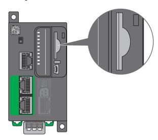
It is possible to set the Write-Control Tab to prevent write operations to the SD card. Push the tab up, as shown in the example on the right-hand side, to release the lock and enable writing to the SD card. Before using an SD card, read the manufacturer's instructions.
