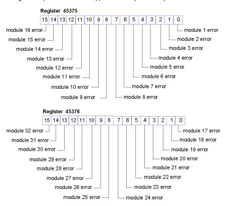
The Emergency Messages registers can be accessed via RTP by writing the following values to the RTP request block:
