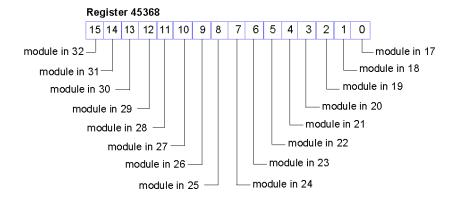
The Node Assembly registers can be accessed via RTP by writing the following values to the RTP request block:
