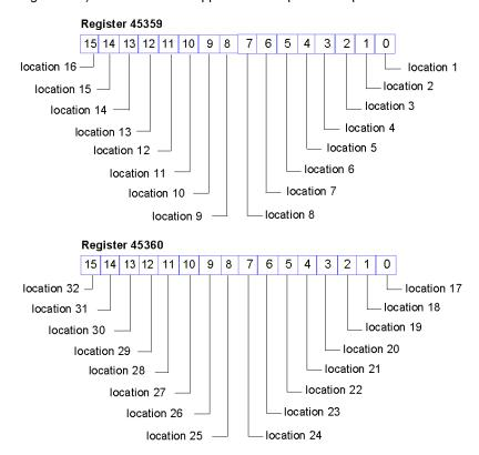
The Node Configuration registers can be accessed via RTP by writing the following values to the RTP request block:
