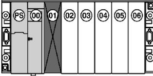
**Installation on extendable rack at address 1 to 7 regardless of the type of processor**
