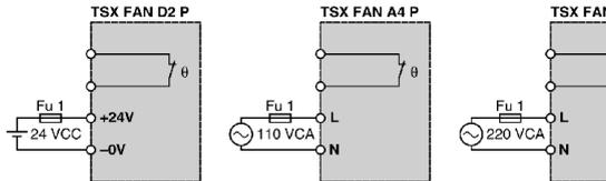
**NOTE:** When using several ventilation modules of the same type, use a common power supply for all the ventilation modules.
