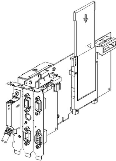
**NOTE:** If the program in the PCMCIA memory cartridge contains the **RUN AUTO** option, the processor will automatically restart in RUN mode after the cartridge is inserted and the PC is turned on.
