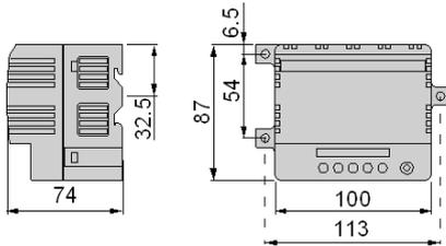
The TSX SUP 10 power supply module must be mounted vertically to optimize the natural convection of air inside the module.
