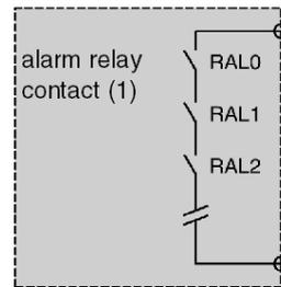
(1) When the PLC station is composed of several racks: set all the "alarm relay" contacts in series (RAL0, RAL1, RAL2, etc.).
