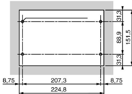
(1) The diameter of the fixing holes must be suitable for M6 screws.
