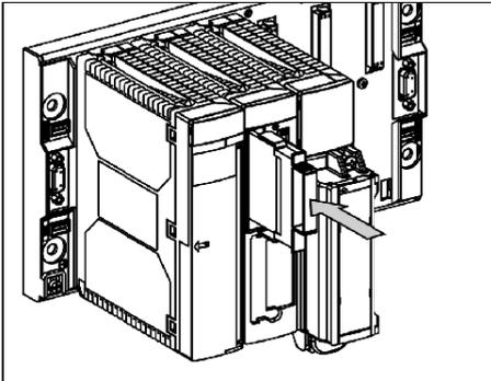
**NOTE:** For TSX 57 1•4/2•4/3•4/4•4 processors, check that the mechanical locating devices are positioned correctly:
