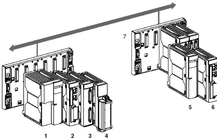
**NOTE:** If the second rack does not contain a processor module, this is a **single** PLC station distributed on 2 racks.
