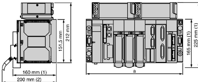
(1) with screw terminal block module,
