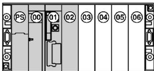
**Installation on standard or extendable rack at address 0 with the Atrium processor**
