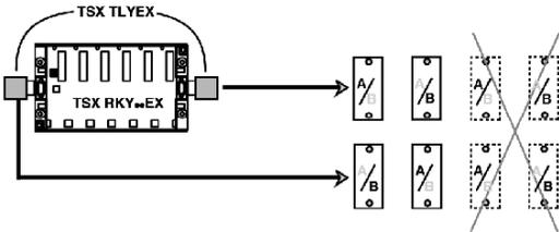
**NOTE:** When a single extendable rack is used, a line terminator must always be mounted on each of the rack's 9-pin SUB D connectors.
