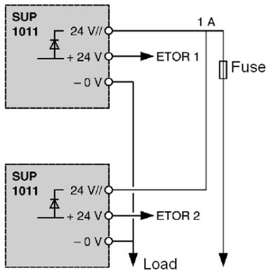
Discrete inputs 1 and 2 on the PLC indicate the loss of one or other of the power supplies.
