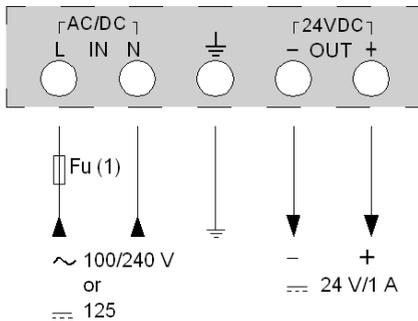
(1) External phase protection fuse: 1A time-delayed 250 V if power supply alone.
