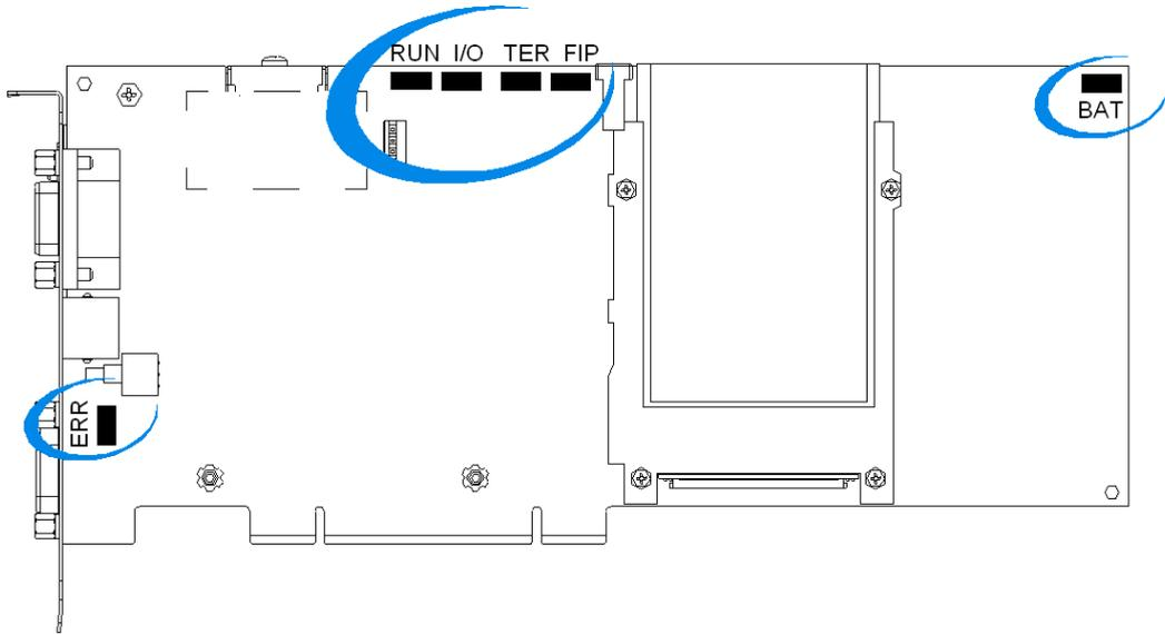
Due to the small amount of space available on the shield, only the ERR LED is visible when the PC housing the processor is closed.
