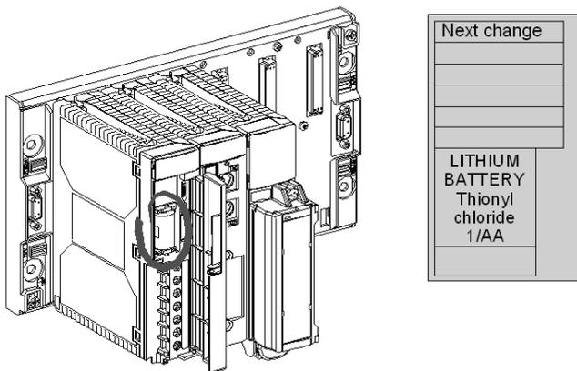
If there is a power outage while the battery is being changed, the processor ensures the RAM memory is saved, as it has its own offline independent save function.
