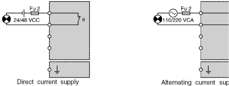
**NOTE:** When using several ventilation modules, the probe contacts shall be serialized.
