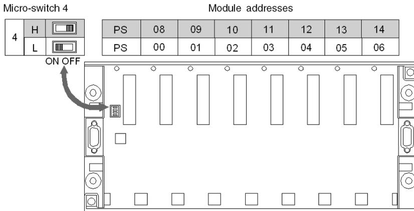
**NOTE:** the grayed-out addresses are only accessible from the programming software
