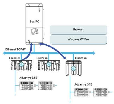
With its built-in Ethernet 10/100 Mbps ports, you can integrate the Box PC into *full Ethernet* architectures, such as Transparent Ready. Transparent Ready devices in this type of architecture enable transparent communication over the Ethernet TCP/IP network. Communication services and Web services permit the sharing and distribution of data between levels 1, 2 and 3 of the Transparent Ready architecture.
