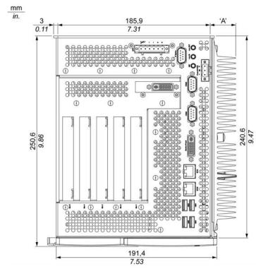
This illustration below shows the dimensions of top view:
