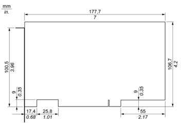
The following figure shows the dimensions of the standard half-size PCIe card:
