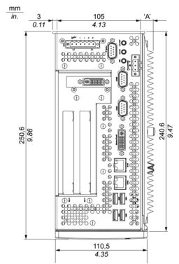
This illustration below shows the dimensions of top view:
