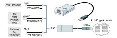
Modbus Plus network with the TSXCUSBMBP converter. This converter is compatible with PCs equipped with CONCEPT, ProWORX or Unity Pro. An example is provided in the drawing below:
