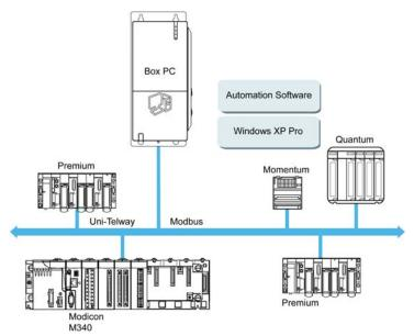
The Box PC terminal with Vijeo Designer automation software can be used in fieldbus architectures such as Uni-Telway/Modbus or Fipway/Modbus Plus.
