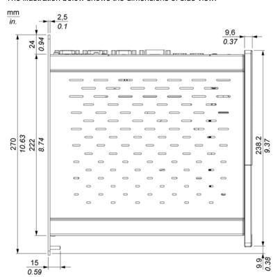
The illustration below shows the dimensions of side view:
