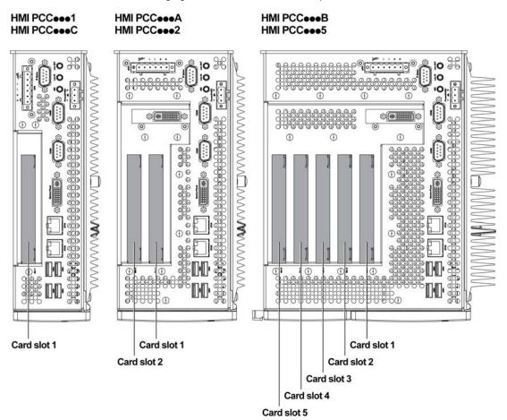
**NOTE:** Take into account the PCI/PCIe card type restriction according to the table below.
