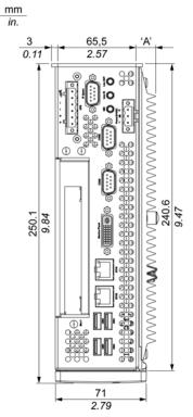
NOTE: Measurement "A" depends on which heat sink is used (see page 56).
