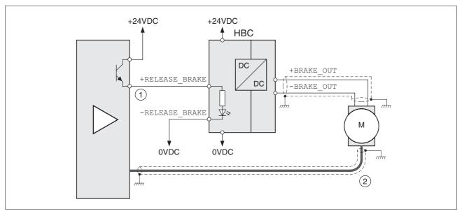
Figure 4.1 Connecting the HBC to the drive and the holding brake
