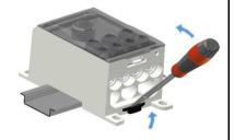
Mounting with screw. Max. Ø 5
