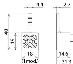
Pin-shaped terminal for EMC-optimised feed-through wiring of lightning current and surge arresters according to IEC 60364-5-53.
