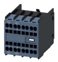
auxiliary switch, on the front, 2 NO, .3/.4, .3/.4, --/--, current path: 1 NO, 1 NO, --, --, spring-loaded terminal, for contactors 3RT2 and contactor relays 3RH2
