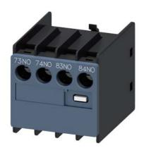
auxiliary switch, on the front, 2 NO, 73/74, 83/84, current path: 1 NO, 1 NO, cable entry from the top, screw terminal, for contactors 3RT2 and contactor relays 3RH2
