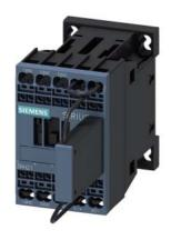
Contactor relay for railway, 3 NO, 110 V DC, 0.7  $\dots$  1.25\* US, with integrated suppressor diode, Size S00, Spring-type terminal suitable for PLC outputs
