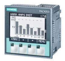
SENTRON, measuring device, 7KM PAC4200, LCD, L-L: 690 V, L-N: 400 V, 5 A, 3-phase, Modbus TCP, optional Modbus RTU / PROFINET / PROFIBUS / DI/DO, apparent/active/reactive energy / cos phi, harmonics: 2.-64., THD, class 0.2 acc. to IEC61557-12 or cl. 0.2S acc. to IEC62053-22, wide-range pwr sup. unit AC/DC, ring cable lug connection
