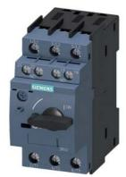
Circuit breaker size S00 for motor protection, CLASS 10 A-release 1.4...2 A N-release 26 A screw terminal Standard switching capacity with transverse auxiliary switches 1 NO+1 NC
