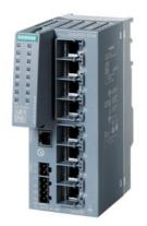
SCALANCE XC208 manageable Layer 2 IE switch; IEC 62443-4-2 certified; 8x 10/100 Mbit/s RJ45 ports; 1x console port; diagnostics LED; redundant power supply; temperature range -40 °C to +70 °C; assembly: DIN rail/S7 mounting rail/wall Office redundancy functions features (RSTP, VLAN,...); PROFINET IO device Ethernet/IP-compliant C-plug slot;
