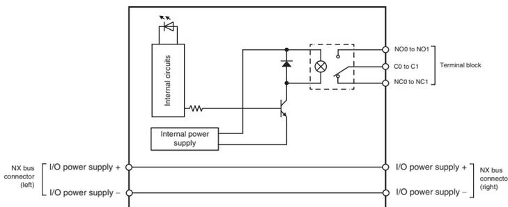
NO0 and NO1 are normal open contacts, and NC0 and NC1 are normal close contacts. You cannot replace the relay.
