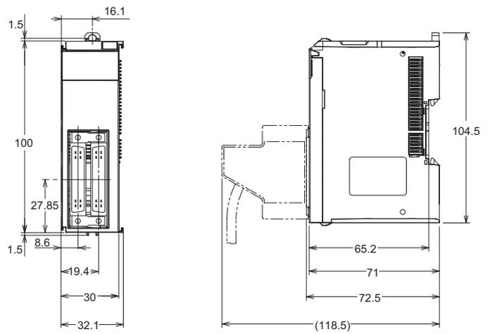
I/O unit with M3 screw terminal block
