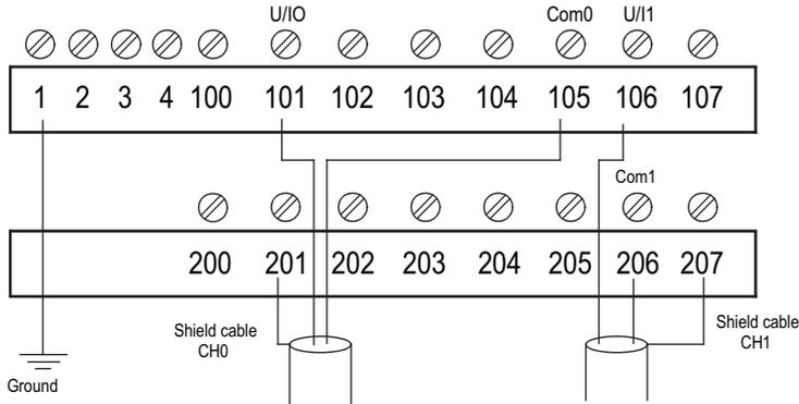
The following table shows the distribution of analog outputs on the TELEFAST ABE-7CPA21 terminal block with a BMX FCA ••0 cable:
