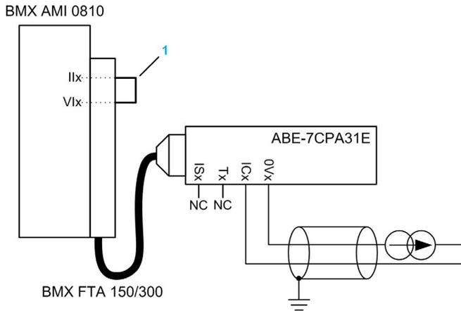
**NOTE:** For the ground connection use the additional terminal block ABE-7BV10/20.
