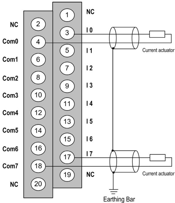
**I<sub>x</sub>** - + pole input for channel x.
