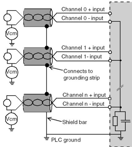
If one or more sensors are referenced in relation to the ground, this may in some cases return a remote ground current to the terminal block and disturbs the measures. It is therefore **essential** to follow the following rules:
