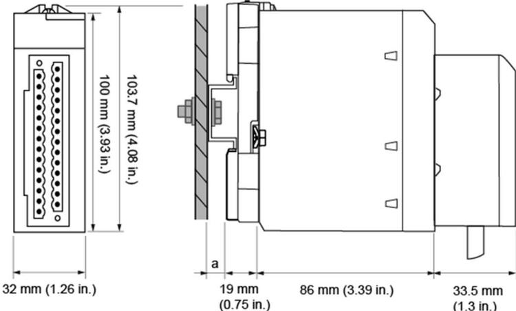
**a** DIN-rail depth: the value depends on the DIN-rail type used in your platform. Refer to *Mounting the Racks (see Modicon X80, Racks and Power Supplies, Hardware Reference Manual)*.
