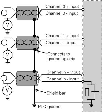
If the sensors are referenced in relation to the ground, this may in some cases return a remote ground potential to the terminal block. It is therefore **essential** to follow the following rules:
