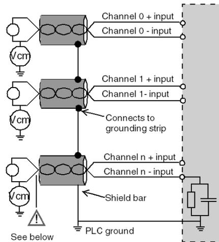
If the sensors are referenced in relation to the ground, this may in some cases return a remote ground potential to the terminals or the FCN connector. It is therefore essential to follow the following rules:
