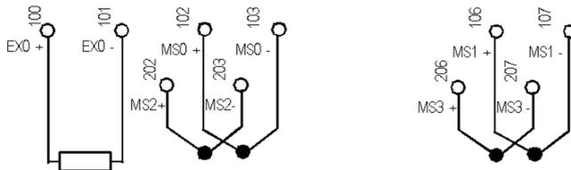
**Legend:** Operating in TC mode with cold junction compensation using a 2-wire PT100 probe.
