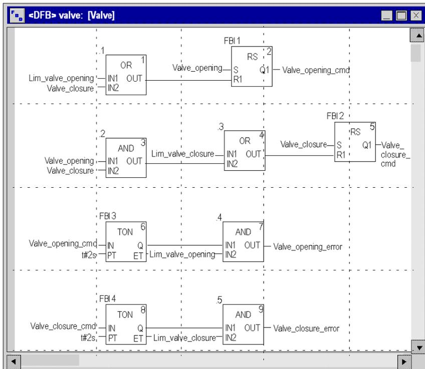
This DFB authorizes the command to open the valve (Valve\_opening\_cmd) when the inputs Valve\_closure and Lim\_valve\_opening are set to "0". The principle is the same for closure, with an additional safety feature if the user requests the opening and closing of the valve at the same time (opening takes priority).
