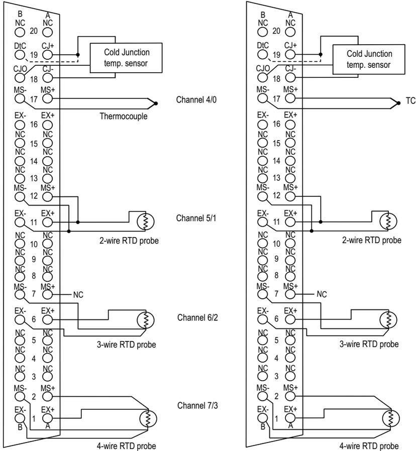
**MS+:** RTD Measure + input / Thermocouple + input
