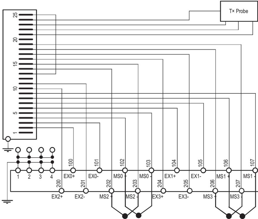
**Legend:** Operating in TC mode with Telefast internal cold junction compensation.
