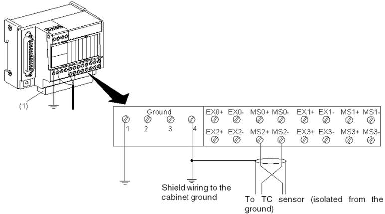
(1) The grounding of cables is facilitated using the ABE-7BV10 accessory.
