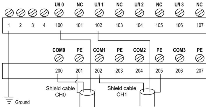
The following table shows the distribution of analog channels on the TELEFAST ABE-7CPA21 terminal block with a BMX FCA ••0 cable:
