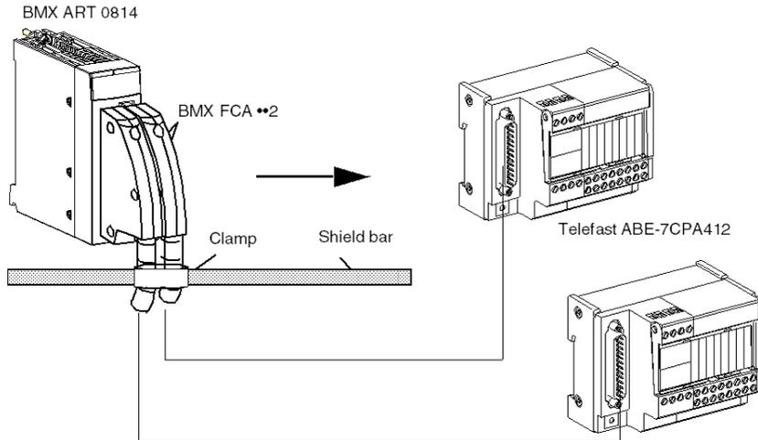
The TELEFAST ABE-7CPA412 accessory is a base unit used to connect 4-channel analog modules to screw terminal blocks.
