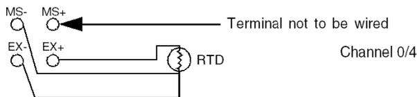
**NOTE:** For the BMX ART 0814 Module, the CJC values of channels 4 to 7 can also be used for channels 0 to 3. Therefore, only one external CJC (*see page 153*) sensor is wired on channel 4.
