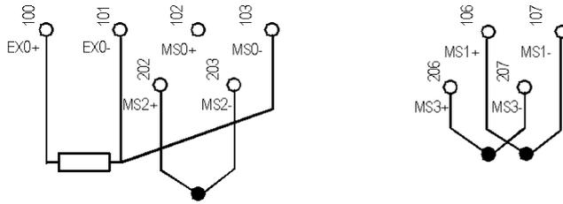
**Legend:** Operating in TC mode with cold junction compensation using a 3-wire PT100 probe.
