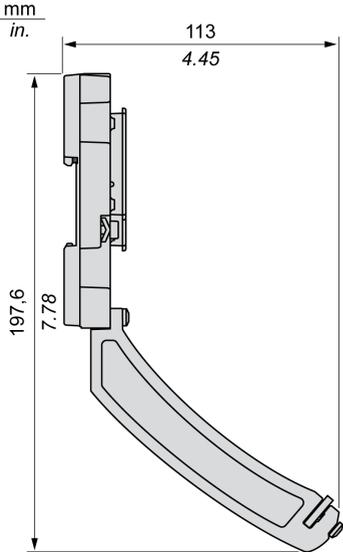
**NOTE:** The overall width equals to the width of the Modicon X80 rack.
