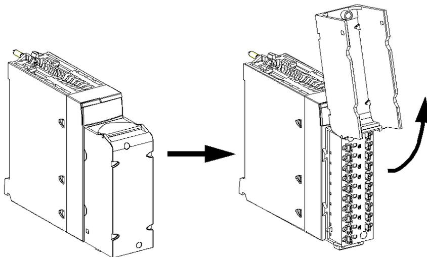
**NOTE:** The connection cable is installed and held in place by a cable clamp positioned below the 20-pin terminal block.
