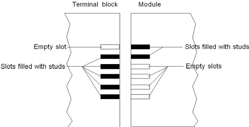
**NOTE:** The module connector have indicators which show the proper direction to use for terminal block installation.
